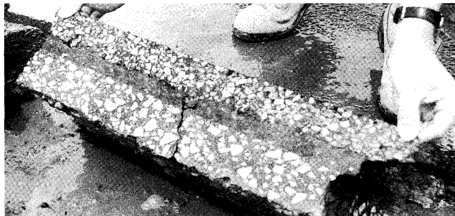
PHOTOGRAPH 9. TEST PIECE CUT FROM STONE MASTIC ASPHALT (SMA 3) TEST SECTION.
