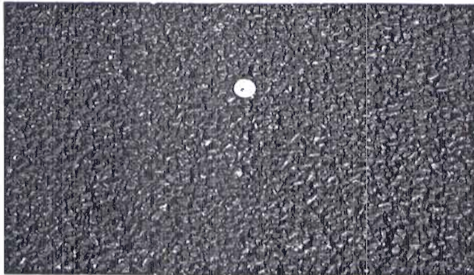
PHOTOGRAPH 8. CLOSE-UP OF STONE MASTIC ASPHALT (SMA 3) SURFACE TEXTURE AFTER FIVE WEEKS.
