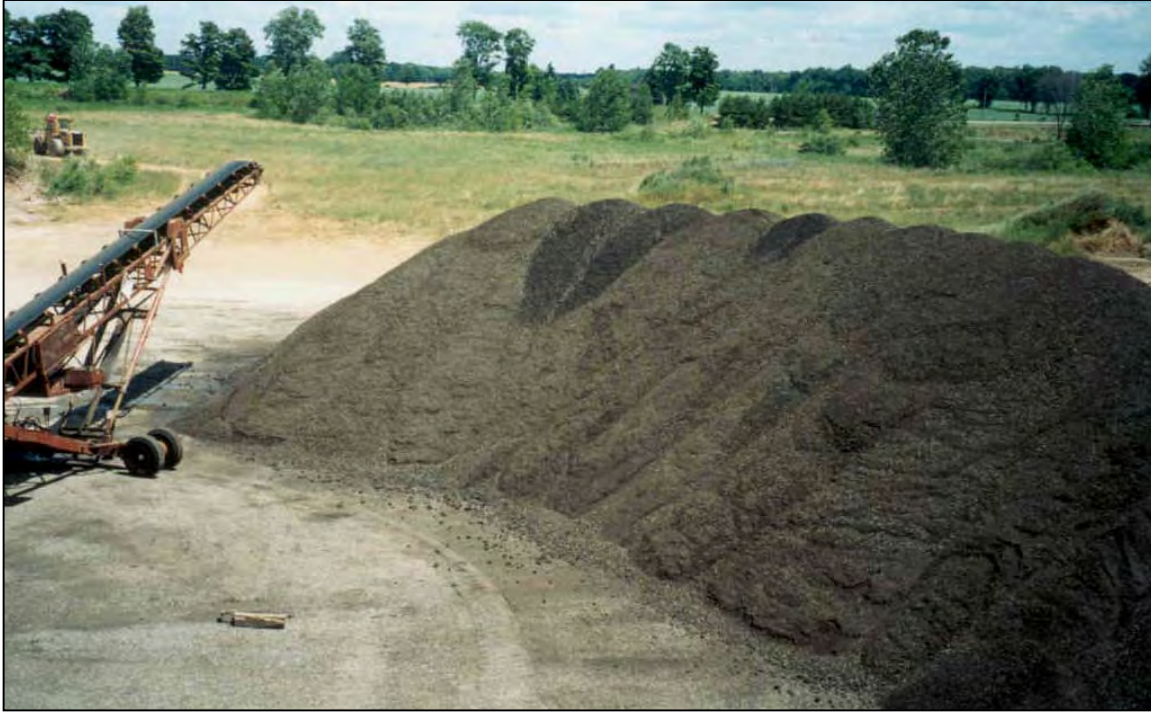
Photograph 8: Stockpiled recycled cold mixture
