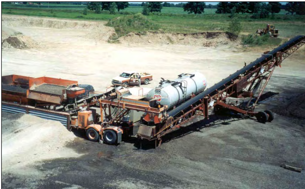
Photograph 7: Two-bin cold mix plant
