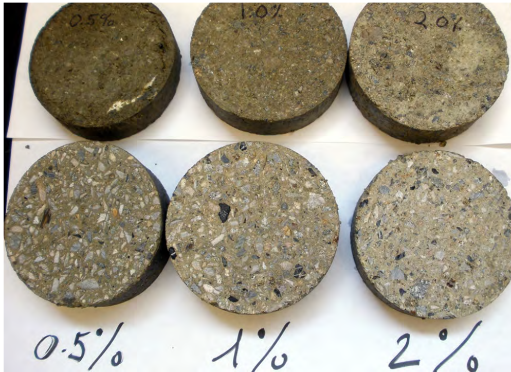
Figure 1. Colour Tones Resulting from Various Percentages of Titanium Dioxide Addition
