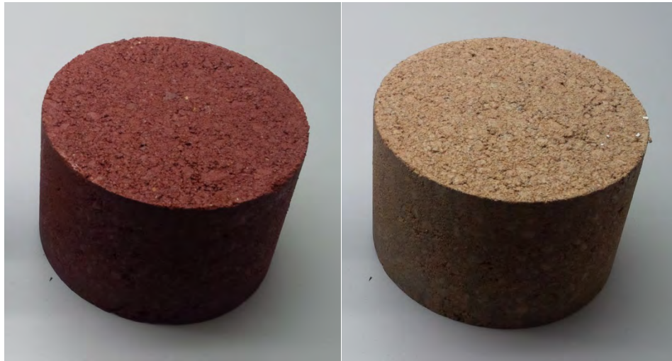
Figure 7. Coloured Paving Materials (Red and Beige) Produced with North American Sourced Components
