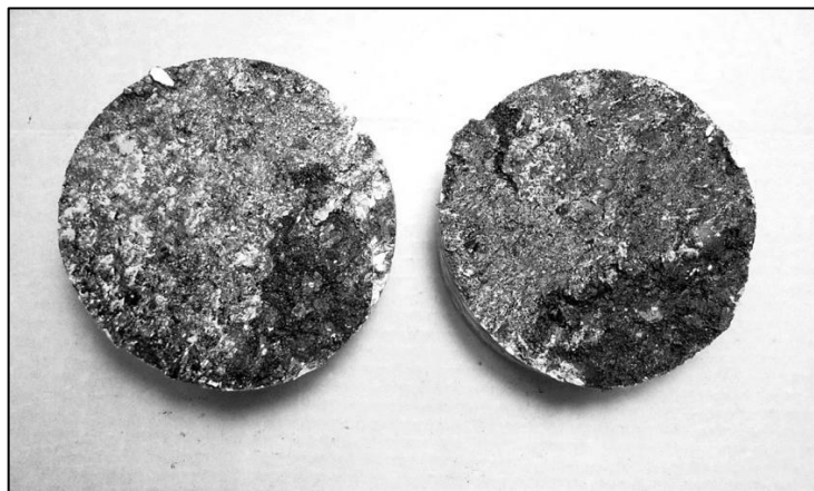
Figure 11. Specimen H3 after shearing; a majority failure mode area is at the interface.
