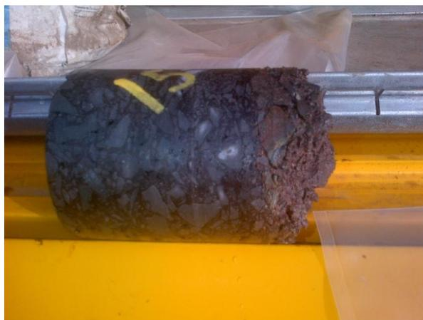
Pic 8.: Two lifts cored with granulars on bottom
