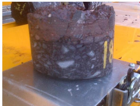
Pic 9: One lift cored with granulars on bottom
