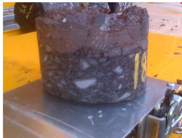
Pic 9: One lift cored with granulars on bottom
